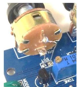
using the controls mounted on the PCB you can wire this set of two pins to the volume control switch via a length of cable.
