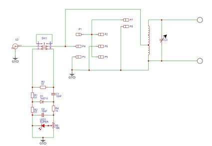
The EFHW uses a resistive SWR bridge with adjustable sensitivity, works well from a few 100mW up to the power limit of the ATU, I recommend keeping the power to QRP levels maybe a little more when matched. Please ignore resistor ref numbers shown on the circuit as they changed on the new PCB.
