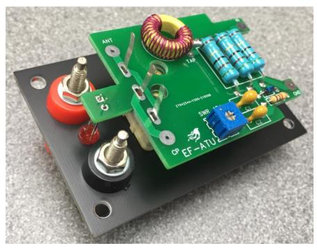
Once you're happy make sure the board is sitting flush on top of the capacitor and solder the three leads in place and trim. Turn the board on its side now and look at the switch, you will most probably need to adjust the single nut on the switch to get it to touch the back of the front plate, this should level up the board. I use a small flat blade screw driver to turn the nut, you don't need to make it tight just get it to touch the front plate.
