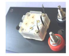
Now Remove the **TOP** nut and washers from the switch (not the bottom nut), drop the LED into the PCB just in front of the switch. Make sure that the long leg of the LED is nearest to the switch (the round hole). DO NOT Solder it yet!
