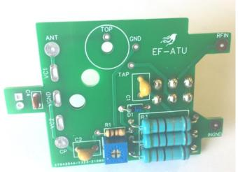
so in a worst case scenario with a short circuit on the output the three will share the full amount of RF power, since we are only using QRP that would be a rated power of 6 Watts but of course we will be only applying power to the tuning bridge for a short time and we hope we will not have a short circuit on the output so these two watt resistors are suitable for our needs. (Also keep the off cuts for now!)
