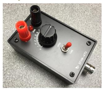
Turn the shaft of the capacitor towards the number 12 on the scale, now fit the supplied knob. The screw should ne nearest the number 1 on the scale.
