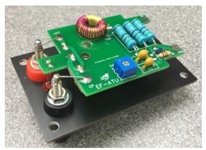
Trim the length of wires so they just fit nicely and solder to the board, the earth tag wire goes to the pad marked GND and the wire from the centre pin goes to the pad marked IN.
