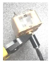
We have now to fit the capacitor to the front panel. First fit the shaft extender, it's a black 10mm long plastic shaft that is secured by a 2.5mm x 12mm screw, be careful here, you can damage the internals of the capacitor by applying to much direct force. Hold the small brass shaft with a pair if cutters while tightening the screw, this keeps any force of the internal parts.
