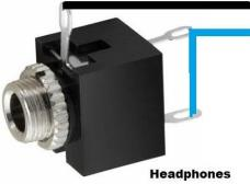
Now connect either a pair of low impendence headphones or small loudspeaker ( $8\Omega$ )
