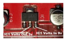
Multimeter Negative Lead to a "GND" position such as a mounting hole. Switch on the Multimeter and ensure battery is connected to the Sudden-2 PCB. Now measure the voltages as per the chart below, if you do not read any voltages make sure the Battery is connected correctly.
