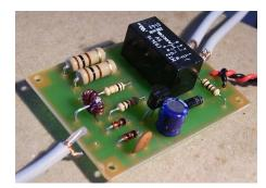
This design was originally provided By Rev. George Dobbs (SK) for the RSGB magazine DIY Radio. Kanga Products were asked to provide a kit of parts for the project. The circuit is fairly straight forward, with the transmitted RF sensed by transformer L1, which is fed to a pair of diodes then to TR1which acts as a high speed switch. *See Fig 3*
