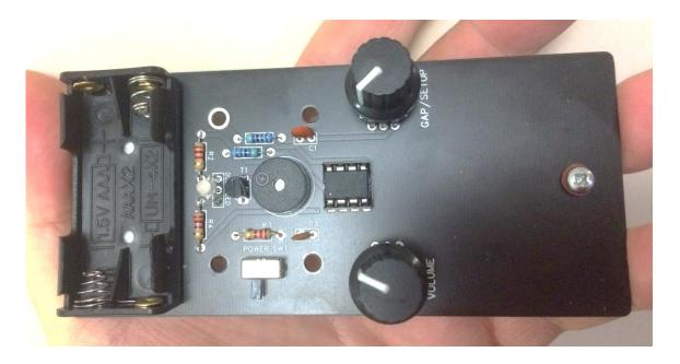
Let's start with the IC socket, make sure you fit it as the layout on the PCB.
