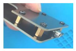
Now drop the top panel onto the base, the black screws should line up with the four fixing holes in the base. Use the four black M3 nuts to attach the two halves.
