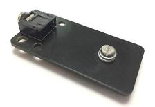
Now fit the bottom contact screw. Find the 6mm Screw (The shortest in the kit) and BEFORE putting it on the bottom board put three of the M3 Steel washers onto the screw (See note at the bottom of this document about setting the gap). Put the screw through the single hole at the one end of the base panel away from the jack socket.
