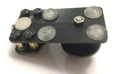
That's it the key is built and ready to test, connect a lead from the keys socket to the radio or oscillator and tap away.
