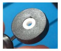
This 1mm plastic washer makes sure the knob is fitted in the centre of the flange.
