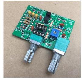
check the back pins are only just protruding and solder them in place. The most common fault with this kit is forgetting to solder the other pins of this control. Once you're happy that the control is fitted as the photo then make sure all five pins are soldered in place. Now fit the second control and angle it the same as the first. This is easier as it's just one row of pins. Make sure you solder all of them this time when happy.
