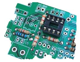
these are ; R2 which is a 10 Ohm resistor and R5 which is 1K8 Now double check that all the resistor values are correct and that you have no bad joints.
