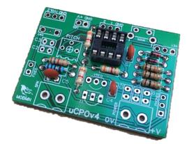
5) Now we will start fitting the capacitors. Fit C1, C4 and C5. All these are 0.1uF disk capacitors and will be marked '104' on the disk. They can be fitted either way round.
