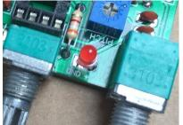
fit the LED is between the two controls. You will see the two holes that it fits in, one hole is square one round. The long leg of the LED MUST go into the round hole. Push the LED in and leave it with about 5mm of leg above the board.
