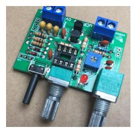
Check the board fitting, at this stage you should not have any problems, the LED legs will fold back, just make sure that they do not short on each other. Now remove the board, we have to wire the sockets.
