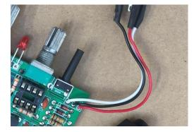
Next to the mode switch you will see three holes marked Key. This is the connection point for the key, the square pad is the GND or common pin for the key and the other two are the left and right paddle connection points.
