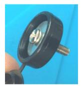
Find the flange, the 3mm white space, the Key top panel and a M3 steel nut.
