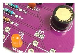
On the MK1 version of this tutor there was a power on LED, I got asked many times if this LED could be made to flash the CW it was sending, well in this MK2 version that's just what it does, you can change the LED to any colour you like, I have supplied a nice Orange LED with the kit. If you look at the LED's leads you will see one leg is longer
