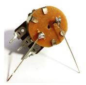
Solder them as shown in the picture below. Use a small piece of heatshrink that came with the kit to insulate one of the wires, no need to shrink this if you don't want to. Solder them to the rectangle behind the control marked SWT
