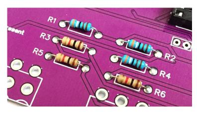
Next fit the 1K Ohm resistors R3, R5, and R6 (first two bands are Brown and Black).
